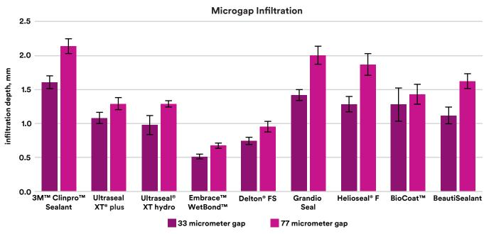
Figure 10: Infiltration depth into 33 and 77 micrometer microgaps. Source: 3M internal data
