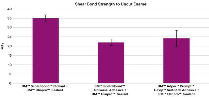
Figure 1: 24 hr shear bond strength of Clinpro Sealant to uncut enamel used with Scotchbond Universal Etchant, Scotchbond Universal Adhesive, or Adper Prompt L-Pop Adhesive. Source: 3M internal data
