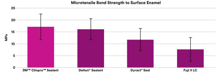
Figure 3: Microtensile bond strength of sealants bonded to buccal enamel surfaces of bovine teeth. Source: Papacchini et al., 2006
