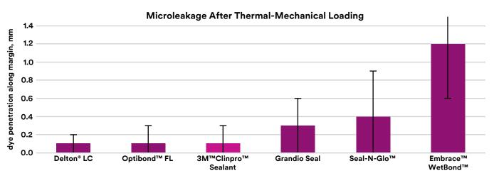
Figure 6: Microleakage after thermal-mechanical loading. Source: Rodriguez et al., 2011.
