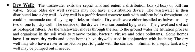
➤ \*\*Dry wells are no longer allowed to be installed as part of a HSTS system. \*\*
