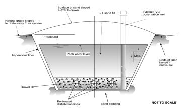
bedrock, a dense soil, or seasonally high ground-water. An ETA system disposes of wastewater into the atmosphere through evaporation, transpiration by plants (usually evergreen trees), and through percolation into the soil. An ETA system is constructed by placing on the surface a layer of gravel over and around your distribution pipes then covering with a mound of sand. Finally vegetation is planted on top of the mound.
