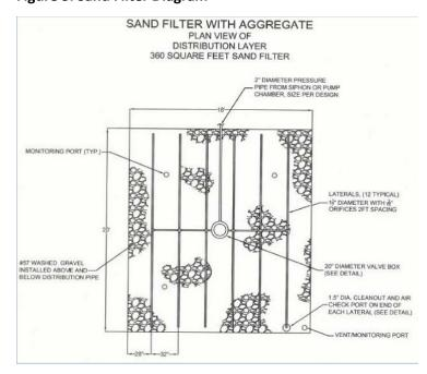
Figure 4: Plan View of Sand Filter Distribution Layer
