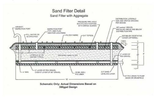
Figure 3. Sand Filter Diagram
