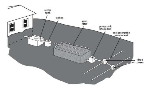
Figure 1. Low Pressure Dosed Sand Filter
